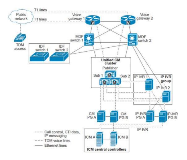
The ICM Server or ICM Central Controller is represented as a single server, but it is actually a set of servers sized according to the Unified CCE agent count and call volume. The ICM Central Controllers include these redundant/duplex servers:
