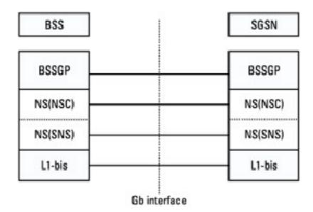
The Gb interface implements a protocol stack in the SGSN and the BSS that includes a User Datagram Protocol (UDP) layer over an IP layer. Data packets are then transmitted between the BSS and the SGSN over a connectionless IP network. The data packets carry information between functional entities in the SGSN and functional entities in the BSS.
