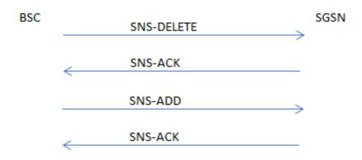
**SNS-DELETE:** The SNS-DELETE PDU is used to delete previously configured IP Endpoints.
