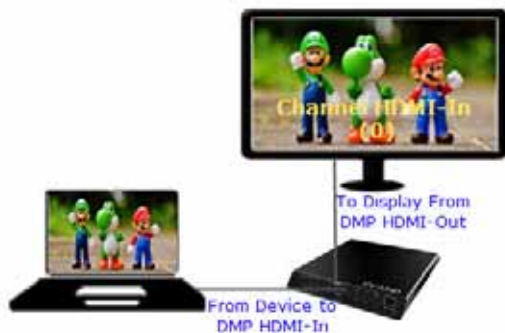
Figure 6 Local HDMI-In Pass-Through to Single TV Display
