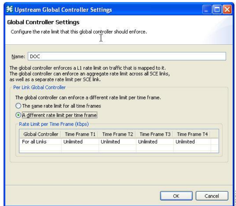
Figure 22: Upstream Global Controller Settings
