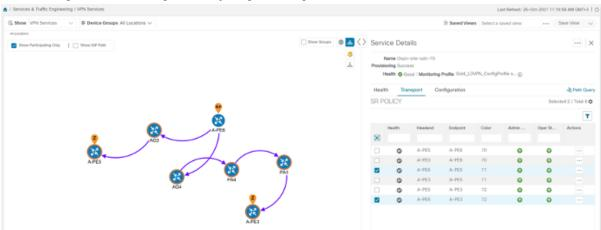
In this example, we are looking at the disjoint paths computed from PE-A to PE-B and from PE-A to PE-C.
