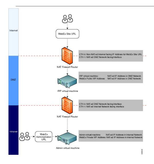
In the diagram, an external user accesses the WebEx site to join or host a meeting. Following a DNS lookup, the IP address for the WebEx site is the NAT public IP address (Eth0). This NAT public IP address is for the external NAT firewall router (Firewall and NAT router 1), between the external network and the DMZ network.
