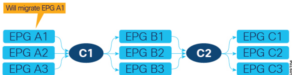
Figure 12: Prepare to begin EPG-to-ESG migration
