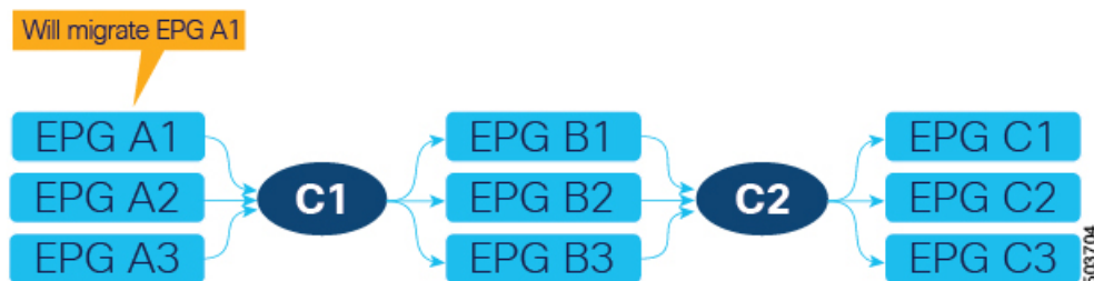
Figure 7: Prepare to begin EPG-to-ESG migration
