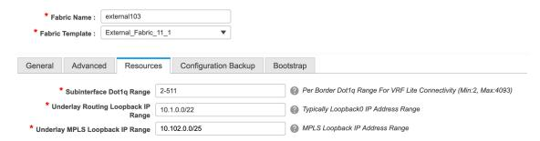
**Underlay MPLS Loopback IP Range**: Specifies the underlay MPLS SR or LDP loopback IP address range.
