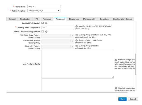
Enable MPLS Handoff: Select the check box to enable the MPLS Handoff feature.
