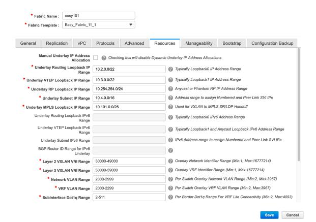
**Underlay MPLS Loopback IP Range**: Specifies the underlay MPLS loopback IP address range.
