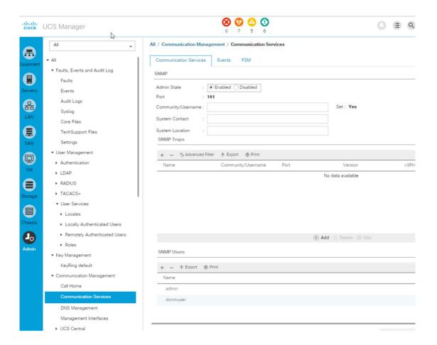
**Step 4** Create a new SNMP user and provide the credentials.
