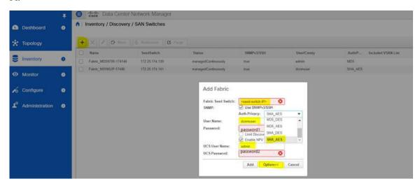
**Step 7** Verify if the UCF FI switches are listed on Cisco DCNM **Web UI > Inventory > Switches**.
