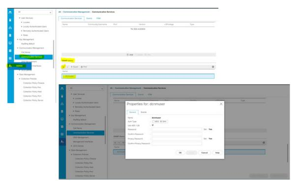
On all the switches in the fabric, you must configure the same SNMP user **dcnmuser** as **network-admin** or **network-operator** with authentication type as SHA\_AES.
