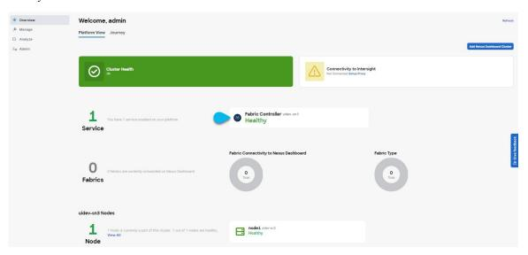
Alternatively, you can log in to any one node via SSH as the rescue-user using the password you provided during node deployment and using the acs health command to check the status:
