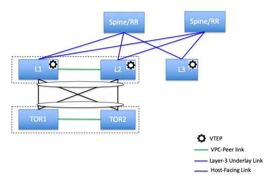
• ToR switches with port channels connected to both the leaf switches. The L1 and L2 switches are connected as a vPC pair.
