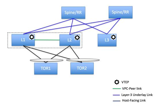
• ToR switches with port channels directly connected to the leaf switches. The L1 and L2 switches are connected as a vPC pair.
