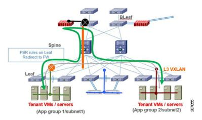
In the previous figure, communication between App group 1 and App group 2 takes place via inter-VLAN/VNI routing in the tenant VRF by default. If there is a requirement where traffic from App group 1 to App group 2 has to go through a firewall, a PBR policy can be used to redirect traffic. The following configuration snippet provides the necessary configuration that redirects the traffic flow
