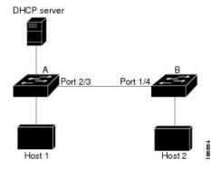
DAI depends on the entries in the DHCP snooping binding database to verify IP-to-MAC address bindings in incoming ARP requests and ARP responses. Make sure to enable DHCP snooping to permit ARP packets that have dynamically-assigned IP addresses.
