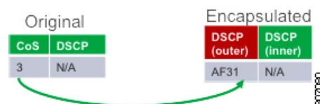
Figure 46: Copy of Priority from Layer-2 Frame to VXLAN Outer Header
