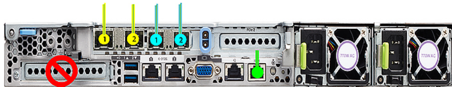
Intel X710 quad-port 10G / Cisco-Intel E810XXVDA4L 4x25/10G
