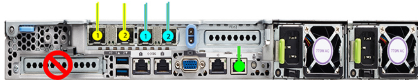
Intel X710 quad-port 10G / Cisco-Intel E810XXVDA4L 4x25/10G
