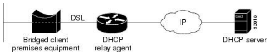
Figure 2 Network Topology Using ATM RBE and DHCP
