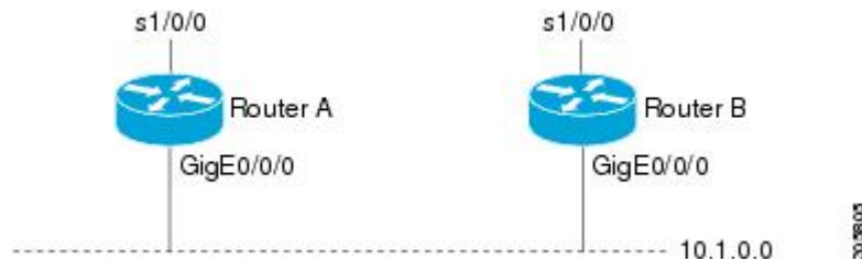
Figure 1: Topology for IP-Routing Support
