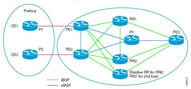
Shadow route reflectors can be both control plane route reflectors and data plane route reflectors.
