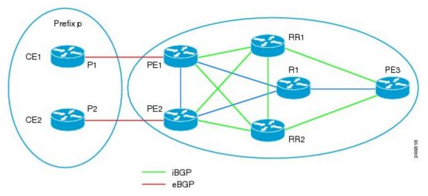
In the figure above, P1 and P2 are diverse paths for prefix p. Assume Path 2 (P2) has a lower MED and higher local preference than P1. The BGP Best External feature on PE1 will make sure that P1 is propagated to the
