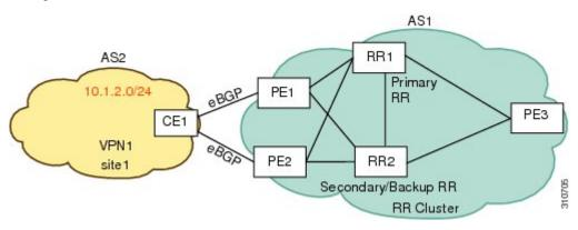
In the following configuration example based on the figure above, RR2 is configured with an additional path, which is a backup path.
