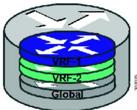
Figure 2: Device Level Virtualization
