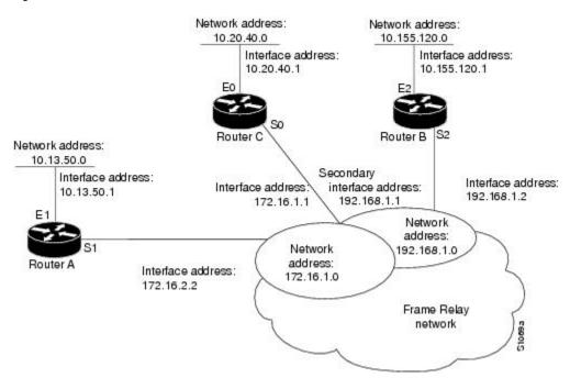
In this example, split horizon is disabled on all serial interfaces. Split horizon must be disabled on Router C in order for network 172.16.0.0 to be advertised into network 192.168.0.0 and vice versa. These subnets overlap at Router C, interface S0. If split horizon were enabled on serial interface S0, it would not advertise a route back into the Frame Relay network for either of these networks.
