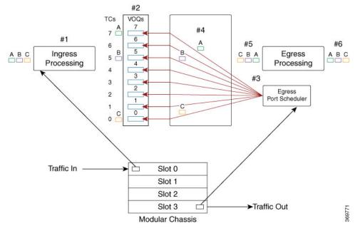
Figure 1: Traffic flow from ingress port on slice 0 to an egress port on slot 3
