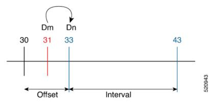
The link delay between 1-2 and 5-6 is normalized to 33.
