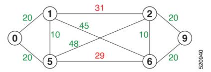
We can normalize the measured latency before it is advertised and used by IS-IS. Consider a scenario with the following:
