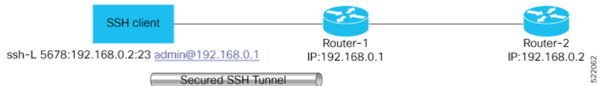
Figure 6: Sample Topology for SSH Port Forwarding
