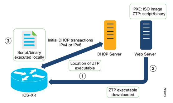
The ZTP process initiates when you boot the network-device with an IOS-XR image. The process starts only on the device that doesn't have a prior configuration.
