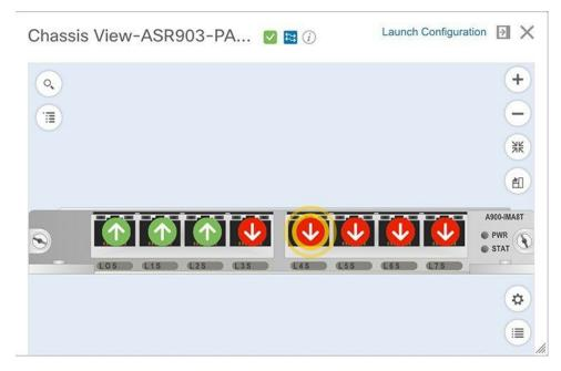
The Chassis View updates, displaying only the line card module that the port resides on and zooming in on it. The port pulsates in the Chassis View to help the user locate it. The badges displayed on the ports in this module indicate the primary status of those port (see Port or Interface States, on page 15). Some elements may be surrounded by colored lines to indicate their state (out of service, pre-provisioned, and so forth). To
