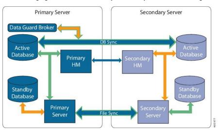
A high availability deployment consists of a primary server and a secondary server with Health Monitor (HM) instances (running as application processes) on both servers. When the primary server fails (due to a problem
