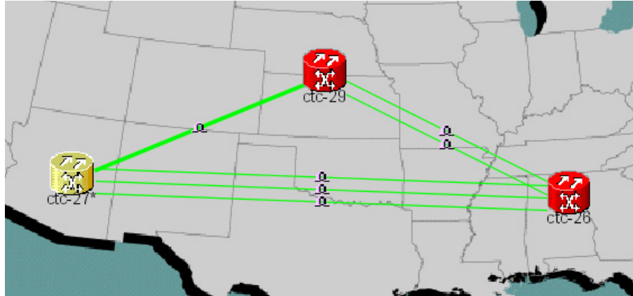
Figure 10-5 Network View with Local Link Consolidation
