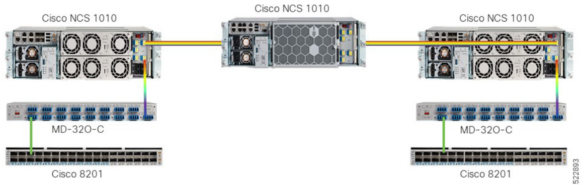
Figure 8: Point-to-point Topology with NCS 1010 Nodes
