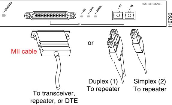
SC-type connectors are used with optical fiber.
