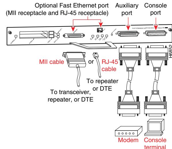
The I/O controller Fast Ethernet port is optional.
