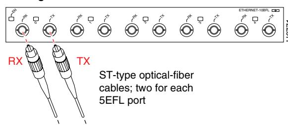
To the appropriate TX and RX ports of the repeater, hub, DTE or other external 10BASE-FL equipment
