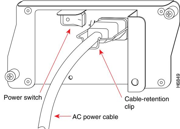
Secure the cable with the cable-retention clip.
