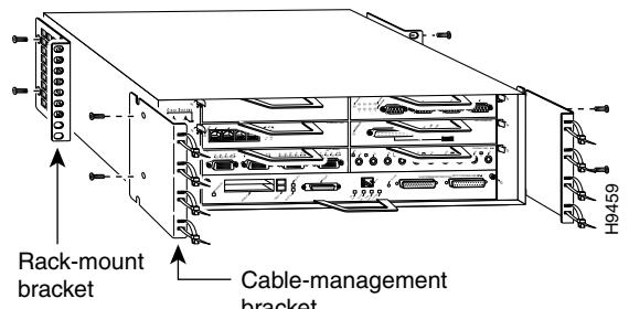
**Step 2** With help from another person, mount the router in the rack using a flat-blade screwdriver and six 10-32 x 3/8 slotted binderhead screws.
