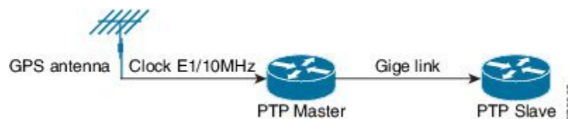
Figure 7: Ordinary Clock Scenario with a GPS Device as Grand Master
