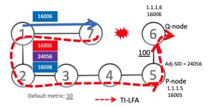
With microloop avoidance configured on Node1, a post-convergence path is computed and possible microloops on the post-convergence path for any destination are detected.
