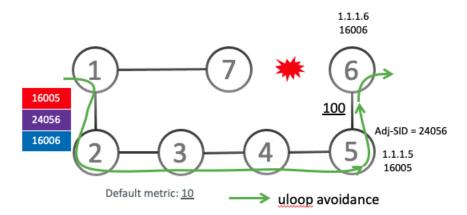
Node1 updates the forwarding table and installs the SID-list imposition entries for those destinations with possible microloops, such as Node6. All nodes converge and update their forwarding tables, using SID lists where needed.
