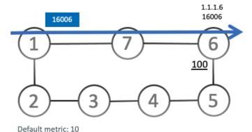
Node1 sends traffic to node 6 (16006) via Node7. Node 7 is configured with TI-LFA to protect traffic to Node6.
