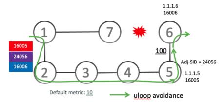
After the RIB update delay timer expires, the microloop-avoidant path is replaced with regular forwarding paths; traffic now natively follows the post-convergence path.
