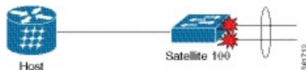
Figure 4: Service-policy on Access Port over Bundle Interface
