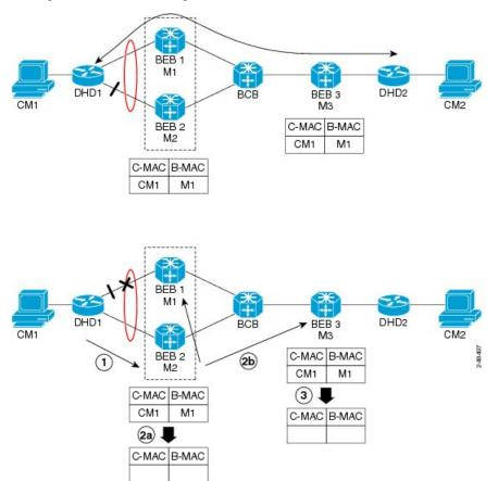
The MIRP has not been defined in IEEE but is expected to be based on the IEEE 802.1ak Multiple Registration Protocol (MRP). MRP maintains a complex finite state machine (FSM) for generic attribute registration. In the case of MIRP, the attribute is an I-SID. As such, MIRP provides a mechanism for BEBs to build and prune a per I-SID multicast tree. The C-MAC flushing notification capability of MIRP is a special case of attribute
