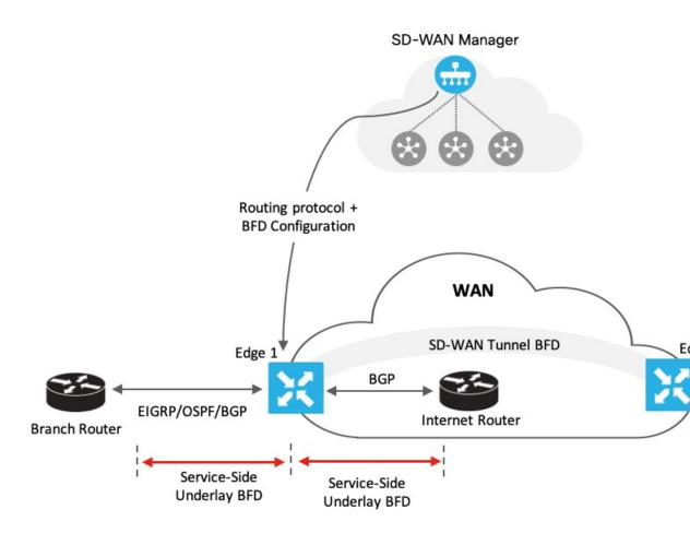
As represented in the image, BFD is configured for a routing protocol through Cisco SD-WAN Manager. Cisco SD-WAN Manager then pushes this configuration to the edge router. In this example, let's assume that OSPF is configured to receive forwarding path detection failure messages from BFD. If there's a physical link failure, OSPF is prompted to shut down its neighbors and restore any routing information it may have advertised to or received from its remote neighbors.
