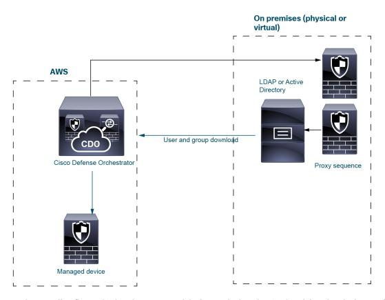
In the preceding figure, CDO and one managed device are deployed to AWS and the other devices are located on premises. These devices can be either physical or virtual; they just need to be able to communicate with each other.
