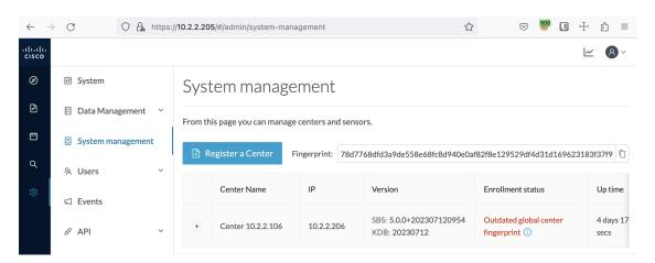
In the Center list, you can see the Center with sync which must be updated with the Global Center's fingerprint.
