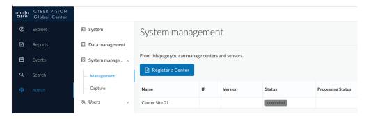
At this point you must switch to the Center's GUI and enroll it to the Global Center.
