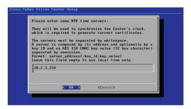
Optionally, add a key ID and an AES A28 CMAC key value separated by a semicolon with the corresponding NTP server.
