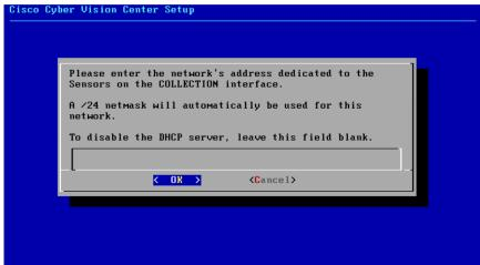
Type the IP address of the Industrial network interface:
