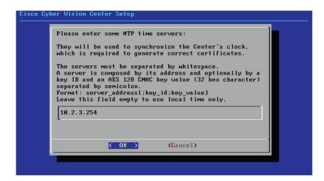
Optionally, add a key ID and an AES A28 CMAC key value separated by a semicolon with the corresponding NTP server.
