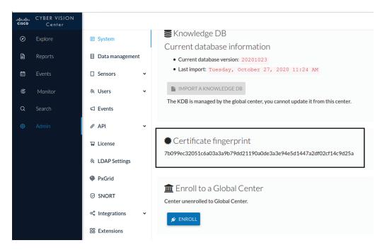
In the Global Center's GUI, give a name to the Center, and paste the Center's fingerprint into the corresponding field.
