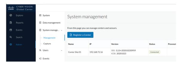
The Global Center and the Center are successfully connected.
