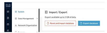
Exports database file limitation is up to 2 GB of data. This avoids side effects related to slow database exports. If the database is larger than 2 GB, you get an error message. In this case, connect to the Center using SSH and perform a data dump. Use the command: sbs db dump.
