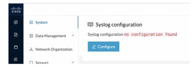
Cisco Cyber Vision provides syslog configuration so that events can be exported and used by a SIEM. The following procedure configures to which machine the syslogs will be sent.
