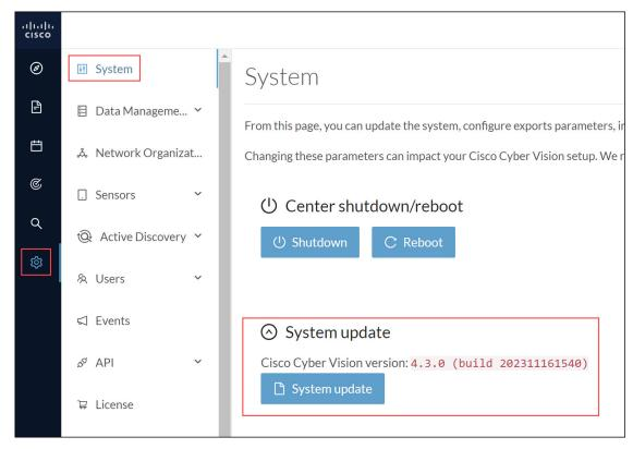
Version releases include a combined update file for the Center, the SENSOR3, SENSOR5, SENSOR7 and the Cisco IC3000 Industrial Compute Gateway. If operating conditions allow, update the Center and all these sensors at once from the GUI. Click **Admin > System**.
