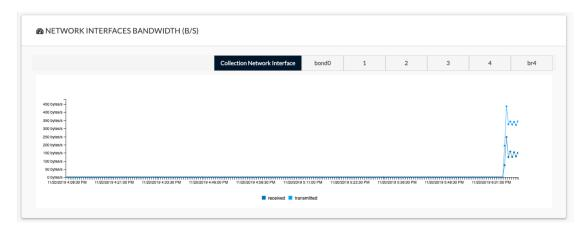
The line charts represent the Collection and Industrial network interfaces bandwidth with the number of bytes received and sent by the Center per second.
