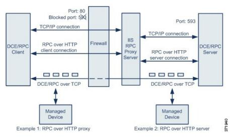
The Microsoft IIS proxy server and the DCE/RPC server can be on the same host or on different hosts. Separate proxy and server options provide for both cases. Note the following in the figure:
