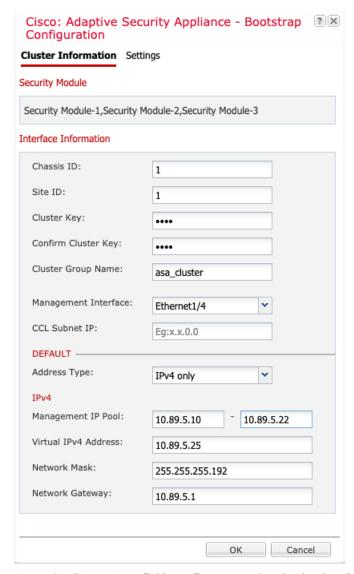
a) In the Cluster Key field, configure an authentication key for control traffic on the cluster control link.
