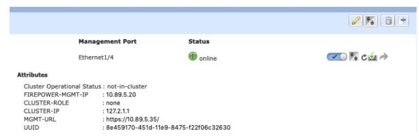
• Disable clustering in the application—You can disable clustering using the application CLI. Enter the **cluster remove unit** *name* command to remove any unit other than the one you are logged into. The bootstrap configuration remains intact, as well as the last configuration synced from the control unit, so you can later re-add the unit without losing your configuration. If you enter this command on a data unit to remove the control unit, a new control unit is elected.
