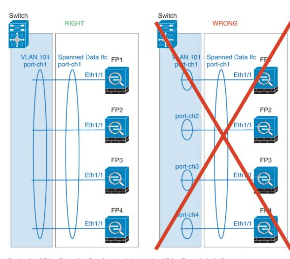
• Device-local EtherChannels—For cluster unit *Device-local* EtherChannels including any EtherChannels configured for the cluster control link, be sure to configure discrete EtherChannels on the switch; do not combine multiple cluster unit EtherChannels into one EtherChannel on the switch.
