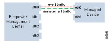
When you use multiple management interfaces, you can improve your performance by dividing the traffic channels over two management interfaces, thus increasing the traffic flow by adding the capacity of both interfaces. One interface carries the management traffic channel and the other carries the event traffic channel. If either interface fails, all traffic reroutes to the active interface and the connection is maintained.
