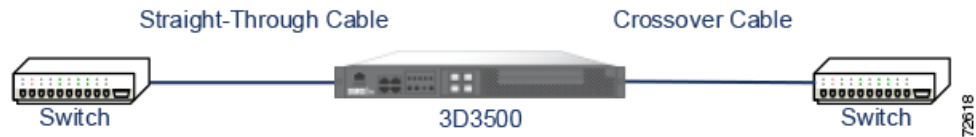
Figure 3-1 Straight-Through Bypass Connection Cabling
