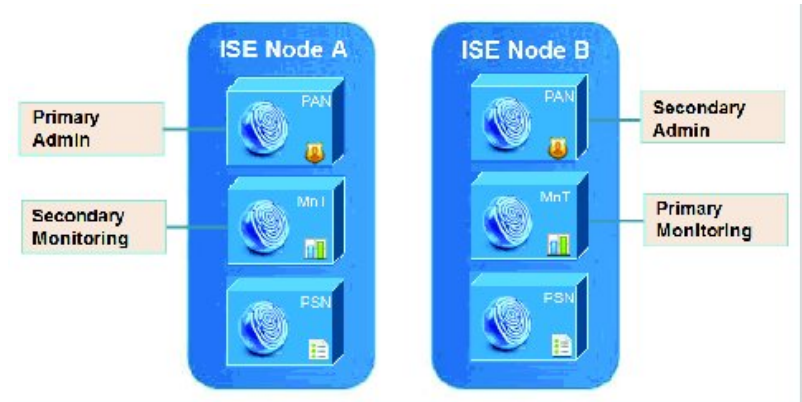
Figure 3: Cisco ISE Two-Node Administrative Deployment
