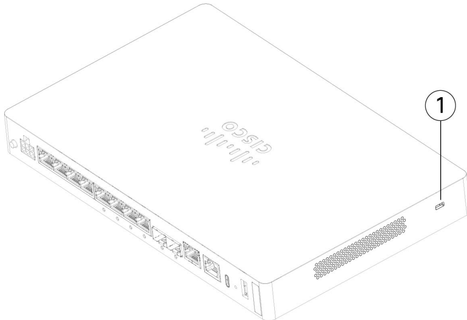
Figure 3: Kensington Lock on the Left Side of Chassis
