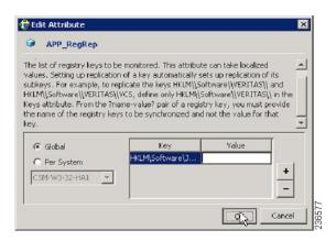
Note Security Manager stores client user preferences in the server registry under HKEY\_LOCAL\_MACHINE\SOFTWARE\JavaSoft\Prefs\vms. The registry replication agent (RegRep) monitors changes to the specified registry location on the active server and synchronizes these changes to a secondary server in the event of a failover.
